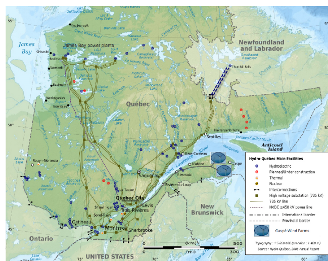
Fig. 13. Province of Quebec power grid with renewable sources in the Gaspé region.
