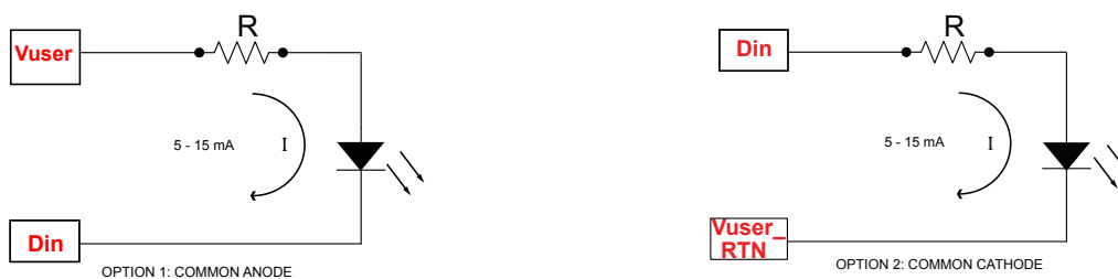
Figure 4: Common Anode (Push) mode and Common Cathode (Pull) mode
