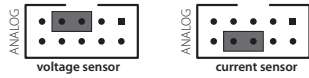
Fig. 7. Jumper positions in order to route one of the measurements to the analog output.
